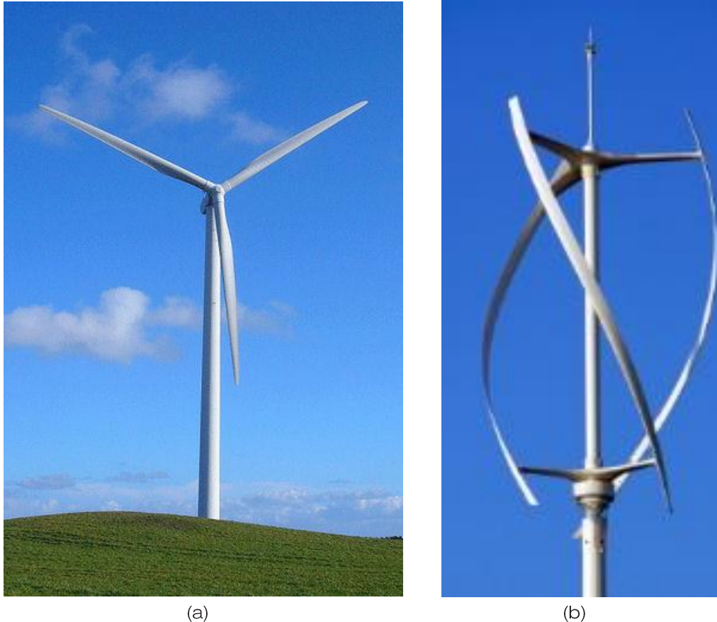
Figure 2: (a) Horizontal axis wind turbines are also known as 'HAWT' (b) Vertical axis wind turbines are also known as 'VAWT'.
