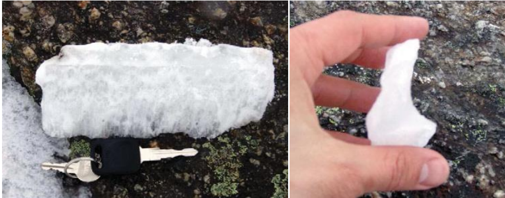
Figure 5: Glaze ice from a wind turbine blade [8]
